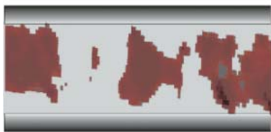
Fig. 1. Schematic of the microreactors. The two model catalytic reactors consist of catalyst layers sandwiched between layers of glass beads for stability. Reactor 1 contains a thin layer of silica gel-supported Wilkinson's catalyst (orange). Reactor 2 contains powdered Wilkinson's catalyst (red) arrayed in various sized clumps to demonstrate a more heterogeneous scenario.
