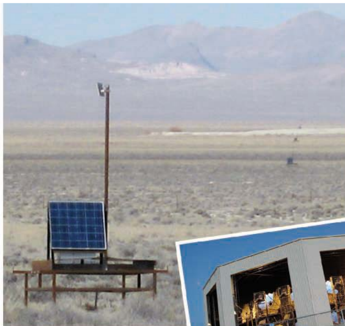
On the range. Spaced 1.2 kilometers apart, Telescope Array's particle detectors stretch across the scrub. Its telescopes (inset) perch on nearby hilltops.
