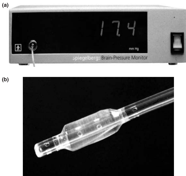
Figure 2.2 (a,b) Spiegelberg compliance monitoring device. Future measurement of ICP may include a continuous estimate of intracranial compliance. Tissue perfusion is more likely to be related to compliance than pressure, and critical volumetric compensatory exhaustion will be detected earlier with this measure. The Spiegelberg device is such a monitor and is currently available
