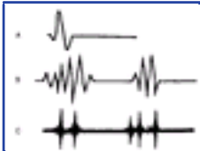
Figure 14-2 These complexes represent the types of signals that the FHR may be required to count. A, ECG; B, Doppler; C, phonocardiogram. Note the complexity of the Doppler signal. To consistently count the same place in the signal complex and avoid artifactually increasing variability, complex signal processing formulas are required.
