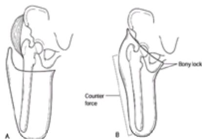
**FIGURE 30-21. A:** The quadrilateral socket is useful for the young child, especially if end-bearing is possible. However, it fails to stabilize the femoral segment in a transfemoral amputation. **B:** This has led to the popularity of the narrow medial lateral socket design, e.g., the ischial containment socket shown here. This design can
