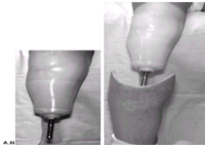
**FIGURE 30-24.** The silicone suspension liners (Triple S socket) have become very popular. The soft silicone liner has a serrated pin incorporated into the bottom of the liner. The patient rolls the liner on the residual limb ( **A**), then inserts the limb into the prosthesis ( **B**). At the bottom of the prosthesis is a socket where the pin locks. It is released by pushing the button on the medial side of the prosthesis.
