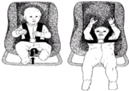
**FIGURE 21.24.** Placing a child in a car seat without locking the crotch strap ( arrow) is a dangerous situation, and can allow serious injury in a collision. (From ref. 201, with permission.)
