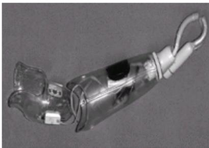
**FIGURE 30-19.** This example of the myoelectric prosthesis was made with a clear socket for teaching purposes. The proximal portion of the socket, which fits on the residual limb, contains the electrodes that pick up the signals from the muscles. This fits into the prosthesis, which contains the electrical and mechanical working parts of the Otto Bock Electrohand.
