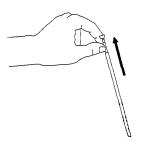
■ To reduce the risk of damage to the antenna, only change its position by adjusting the black plastic base
