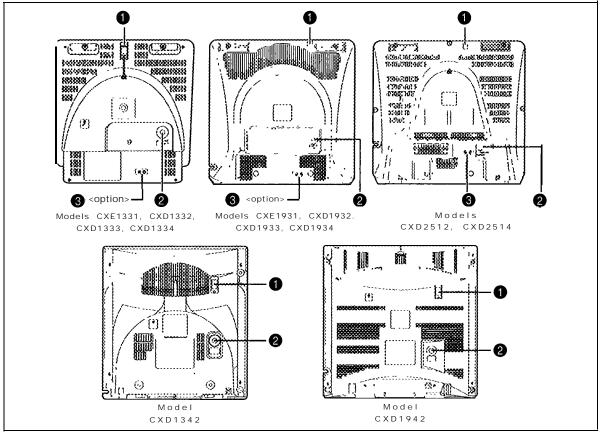
1 VHF Antenna Mount Mount the VHF rod antenna here See page 2.1
