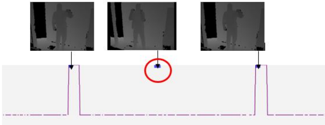
Figure 7. An example of using VGB for verifying correctness of tagging. The analysis indicates that the detector detected two gestures (indicated by the two purple peaks), but three gestures were tagged (indicated by the horizontal blue lines). Visual inspection of what the person actually did indicates that the detector is actually correct, and the tag in the middle is incorrect.
