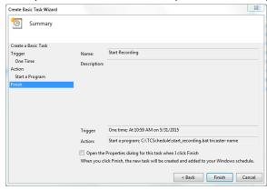
11. When you finish, you will see your task listed. Make sure you create one task to start recording and another task to stop recording. The TriCaster must be sitting in 'Live' with the recording options all configured. When the task time occurs, it will run the script that will trigger the TriCaster to start or stop recording.
